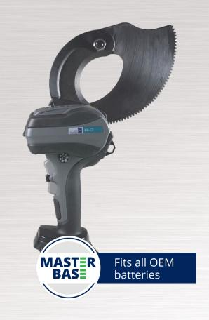
The cable cutter precisely and quickly cuts non-armoured Al-cable of up to NAYY 4 x 240 mm<sup>2</sup> as well as Cu cable up to NYY 4 x 185mm<sup>2</sup> with cutting  $\emptyset$  up to 65 mm. In power supply and cable processing, this lightweight and ergonomic tool convinces with its sickle-shaped cutting geometry.
